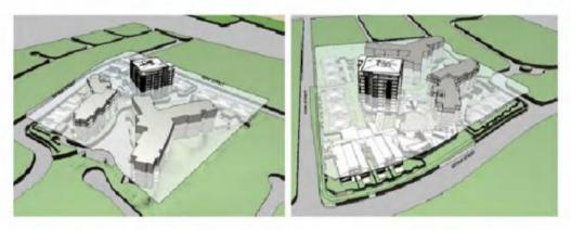
3D models of the proposed development showing the 15.5 metre height control represented by the white coloured plane in relation to proposed Building B and existing approved buildings represented by the two buildings shaded in grey.
